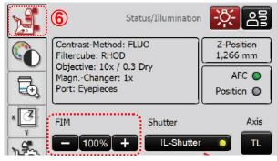
6 On the Touch Screen use the tab to confirm the current FIM (Fluorescence Intensity Manager). The brightness is adjusted in 5 defined increments.
