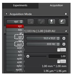
m-2. Following panel will open according to the selected mode. Define the "Duration"(whole acquisition time) and "Time interval"
